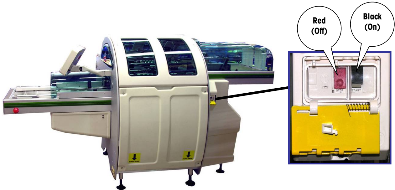
Main Power Switch
