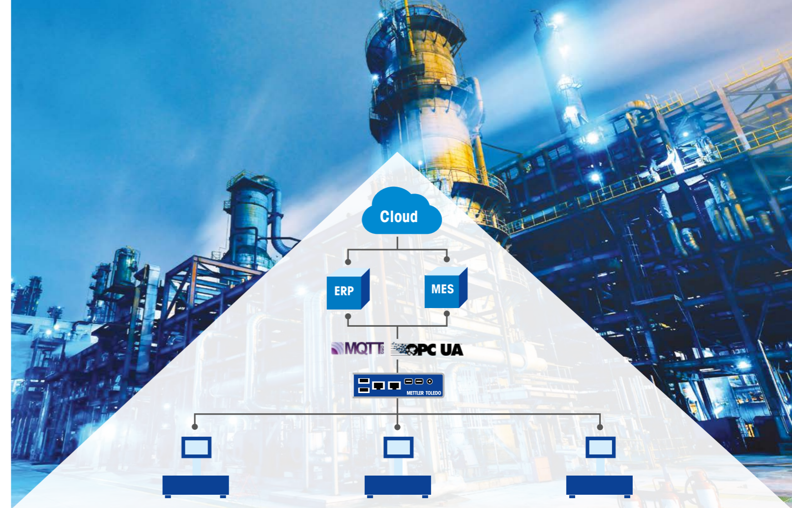
One IIoT Gateway can connect up to four scales to MES, ERP or cloud.
